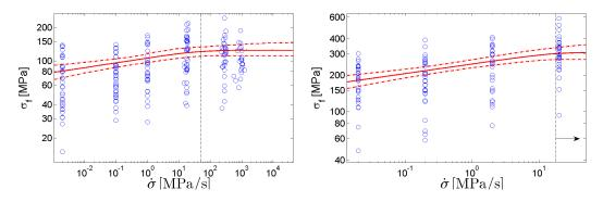
Fig. 2. Results for the data sets RB-data (left) and GS-data (right). Experimental data ( $\circ$ ) together with the median  $\sigma_o$  predicted by FBM (-) and a 95% confidence interval ( $\cdots$ ) are shown. FBM detects where inert strengths are observed; the start of the plateau area is indicated by (--). Note that the RB-data shows a pronounced saturation region, while for the GS-data the plateau is correctly found to lie to the right of the measurements.
