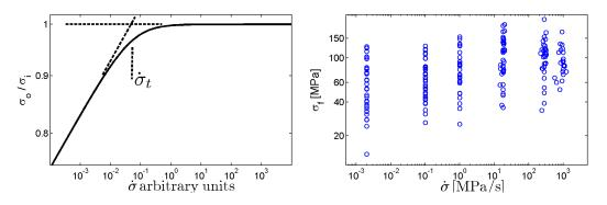
Fig. 1. The left plot shows the dependency (3) between loading rate  $\dot{\sigma}$  and characteristic failure strength  $\sigma_o$  with asymptotes (5). For materials with small Weibull parameter it can be hard to localize the plateau region from experimental data as shown by the right plot (RB-data, see Sec. 4 for details).
